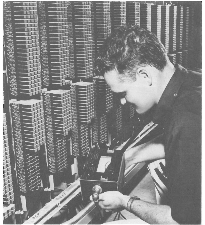
Delcon Model 4910 Open Locator is used to locate "open" faults in paired or single conductor cable. Sturdy five-pound instrument gives operator reading in feet up to 100,000 feet away with an accuracy of \pm one percent.
